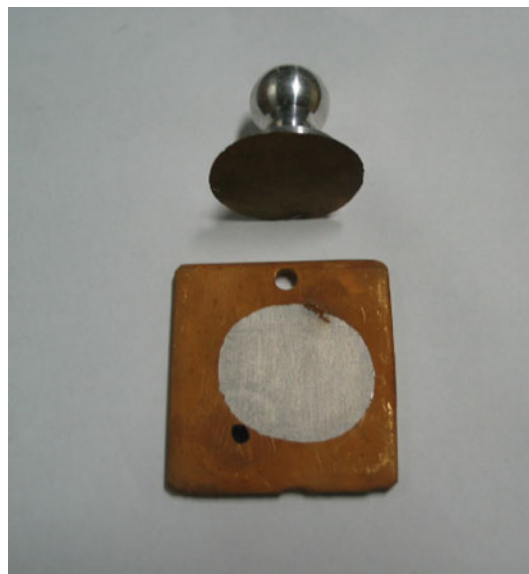
Fig. 9 Test sample and dolly after pull-off adhesion test
